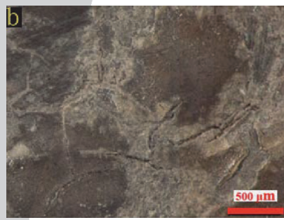
圖9 Return from the Front 表面皂化霧白樣貌。圖片來源：Aviva Burnstock. "Taking Different Forms: Metal Soaps in Paintings, Diagnosis of Condition, and Issues for Treatment," p.246.
